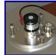
SOLAR RADIATION SENSOR
