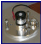
SOLAR RADIATION SENSOR
